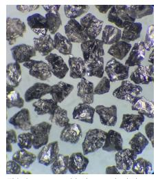
This is a strong blocky tetrahedral or octahedral crystal, with well developed faces and sharp cutting edges, for use in metal bonds and vitreous bonds, for the grinding, sharpening and honing of high-speed steels, superalloys, and cast irons over 45 HRC.
