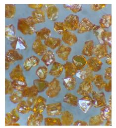
This amber colored crystal has an angular yet semi blocky shape. This allows for high thermal stability, medium to high strength, good adaptability and prolonged tool life. Ideal in single layer bonds, as well as metal and vitrified bonds.
