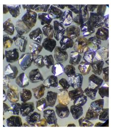
This is a high strength, macrofracture product, ensuring constant sharp cutting features. the crystal morphology between tetrahedral and octahedral enhances bond retention.
