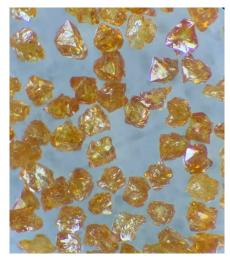
This is an amber colored crystal with a highly angular face rather than a blocky shape. This shape, combined with its high thermal stability and medium strength, makes it a highly versatile grit in wheel production using, vitrified, metal and electroplated single layer bonds.
